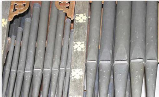
“Diapasons” are flue pipes and represent the basic organ stop. You can mix different lengths of diapasons, for example 8’ and 4’, to give a fuller, characteristic pipe organ sound. Several diapasons played together are known as a “diapason chorus” – a very common sound of the pipe organ.
